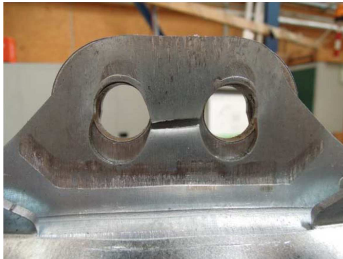
Figure 39: Failure by block-tearing at \varnothing 16 holes
