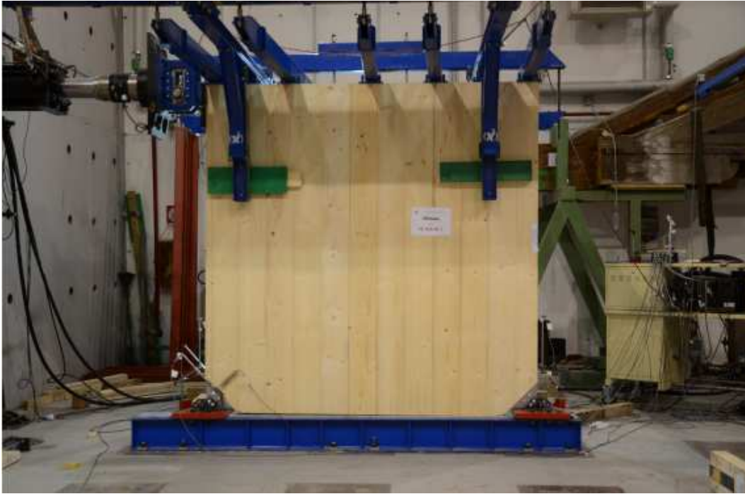
Figure 19: Single panel test set-up
